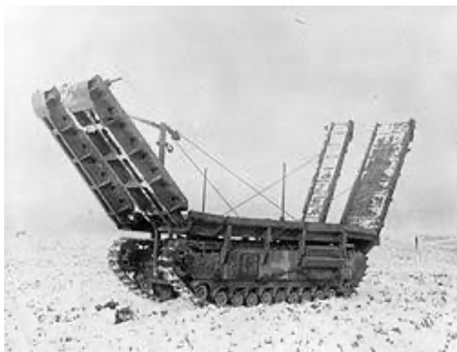
One of Hobart's 'Funnies'. A section of bridge built on a tank chassis
